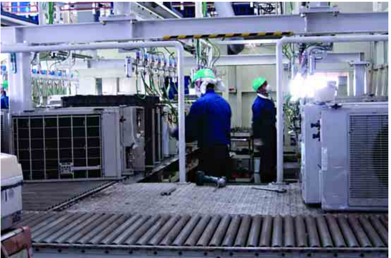
Exhibit D.16 Air conditioner disassembly at METEC
