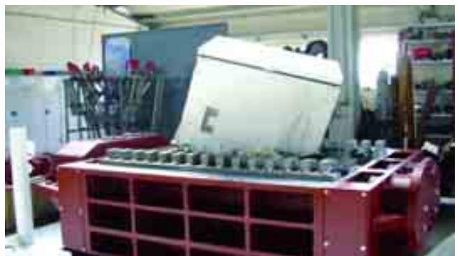
Exhibit 8.13 Twin-shaft shredder (German system)
