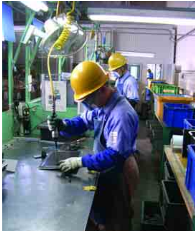
Exhibit D.22 Laptop disassembly at Green Cycle plant
