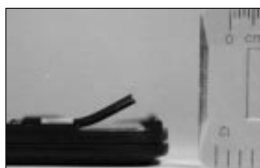
Figure 2: Triggered NiTi actuator displacement for product separation
