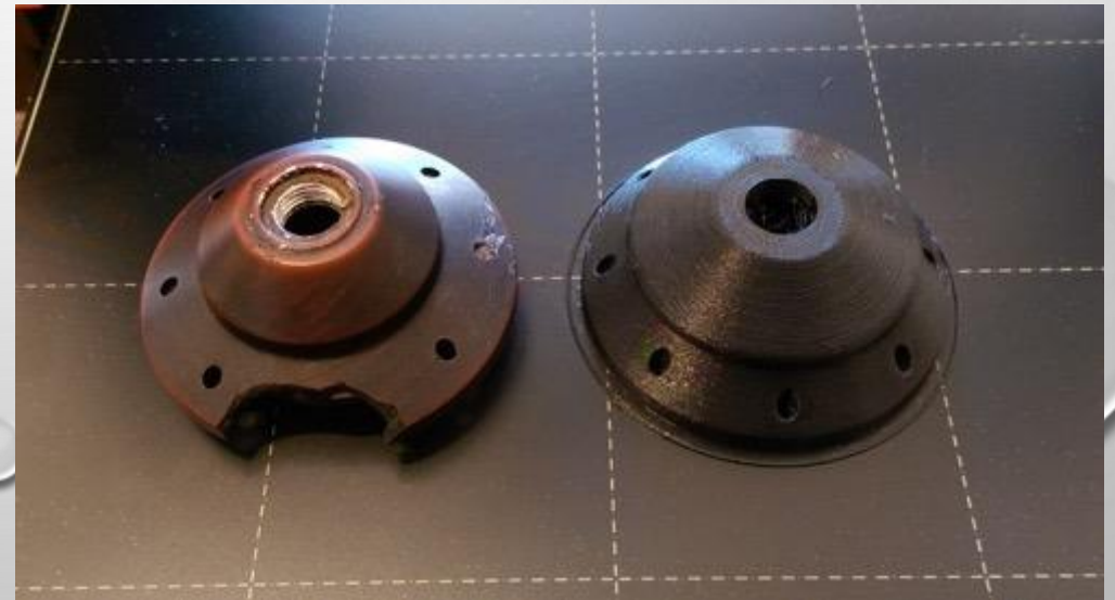
Old and newly created 3D printed part
