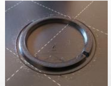
Glass shade 3D printed securing ring
