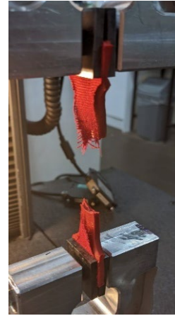
Figure 3.4: A HideBio Tech sample after failure. The woven fibrous backing has snapped and then the main leather-like material has extended a lot before tearing near the change in cross-section
