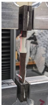
Figure 3.1: A Piñatex sample after failure. The backing has snapped and then the pineapple leaf fibres have pulled out from each other.
