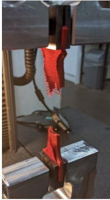
Figure 12.1: A Hide BioTech sample after failure, indicating the elongation achieved before total failure. The woven fibrous backing has snapped and then the main rubbery material has extended significantly before tearing near the change in cross-section.
