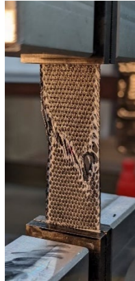
Figure 12.2: A Bananatex sample after failure. The woven fibres and adhesive backing have sheared near the centre of the sample.
