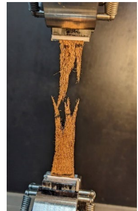
Figure 12.4: A BarkTex sample after failure. Bunches of fibres have pulled out from each other, with the failure happening near the top grip that was in motion.
