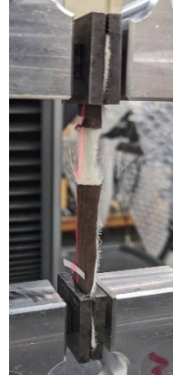
Figure 12.3: A Piñatex sample after failure. The backing has snapped and then the pineapple leaf fibres have pulled out from each other.
