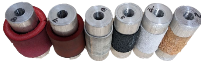
Figure 9: An image of the six rollers with the material adhered, pictured after the abrasion testing.
