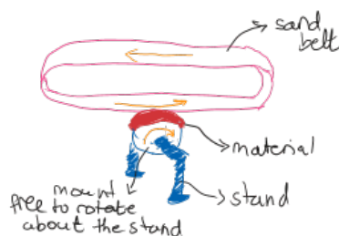
Figure 7: A rough sketch of the initial plan for an abrasion testing rig.
