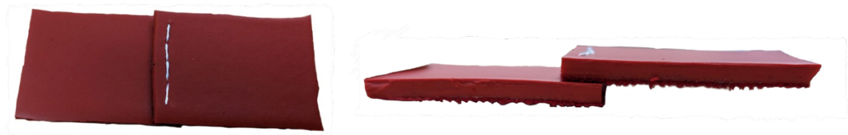
Figure 5: Images of the seam tensile testing sample from both above and the side.
